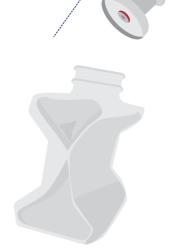
Pull out the **PUMP INSERT**
